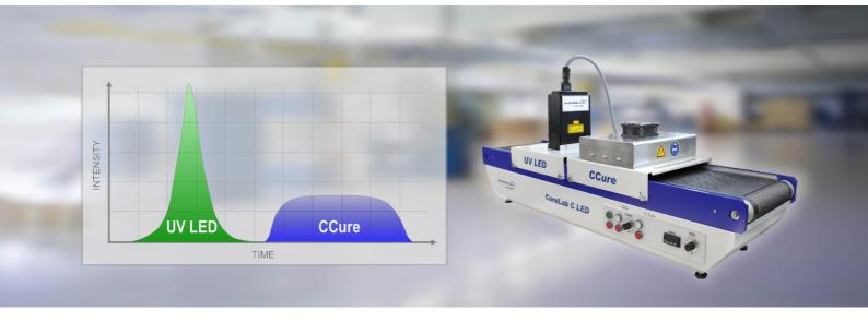
The combination of two innovative UV sources is the special feature of this conveyor belt dryer. The powerful UV LED dryer with it's longer wavelength ensures good deep curing and adhesion of the ink to the substrate. The short-wave UVC radiation of the CCure module causes a forced surface curing.
