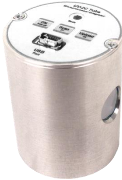
Fig. 13: UV sensor that, in a bottle printing machine, measures the irradiance and the doses of several UV medium-pressure lamps in one pass. Two spectral bands are measured. The measured values are stored internally and can be displayed on a PC as a measurement graph. In this case, the sampling rate is 200/sec. The installed battery can be recharged via a USB cable.
