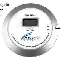
With regular measurements it is therefore possible to anticipate the time and minimum UV dose needed to avoid uncured products. UV lamps can then be cleanded or replaced at the right time, i.e. not too soon to save costs and not too late, to prevent curing problems.
