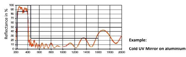
Spectral specification, AOI = 45°. Measured with planar substrate.
