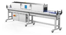
**Function:** The empty cans, jars and packaging to be sterilized are placed on the inlet conveyor belt of the UVC system. The UV disinfection takes place automatically during the run, dry and without additional chemicals. The filling then takes place immediately.
